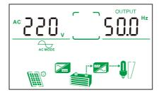
2)Mains working mode (Has PV input, the mains and the PV simultaneously charge the battery)
