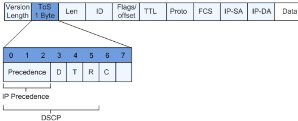
0 to 2 bits are Precedence fields representing the 8 priorities of message transmission ranging from 7 to 0 from high to low, with either Level 7 or 6 as the highest priority that is generally reserved for routing or updating network control communication. User-level applications only have access to Level 0 to 5.
