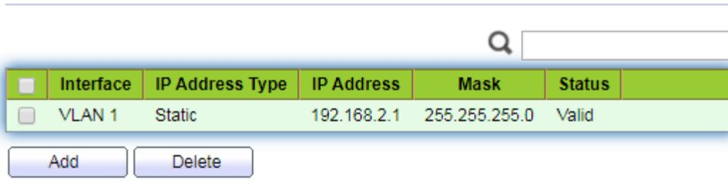
The screenshot shows a web interface for configuring IPv4 interfaces. At the top right, there is a search icon and an empty search box. Below this is a table with the following columns: Interface, IP Address Type, IP Address, Mask, and Status. A single row is visible in the table with the following data: VLAN 1, Static, 192.168.2.1, 255.255.255.0, and Valid. Below the table, there are two buttons: "Add" and "Delete".
