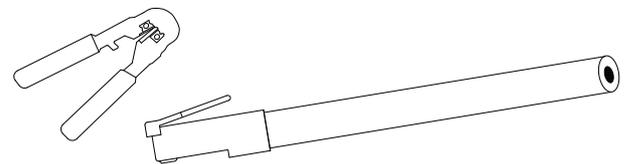
4. Connect RJ45 plug with joint sleeve, and tighten up sealing, sealing nut and joint sleeve.
