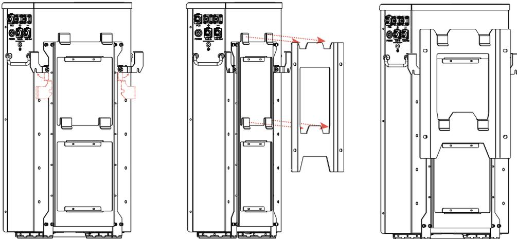
3. Rotate the left latch rightward until the notch locks limiting pin, and rotate the right latch leftward until the notch locks limiting pin too.
