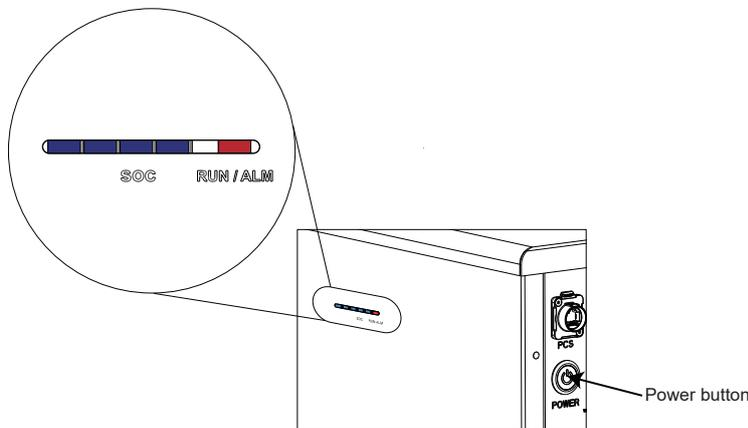
RUN and SOC indicators turn on and indicate correct state. The battery is powered on successfully.
