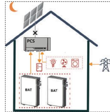
Battery powers loads at nighttime when there is no PV. If battery energy is insufficient, it can empower loads together with grid.
