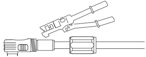
4. Tighten up sealing, sealing nut and joint sleeve.
